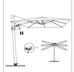
6. Assemble the crank handle to the hole, operating the handle can make the cover turn on the right or left.
