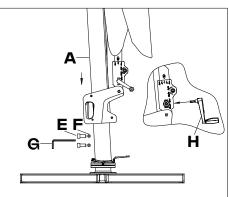
3. Put the parasol (A) on the base and align the holes, then use the 6# wrench (G) to screw the bolts(E) and washers(F). ATTENTION:Make sure the parasol always straight during the assembling process.
