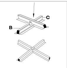
1. Assemble the cross base 1&2(B&C) on a horizontal position.
