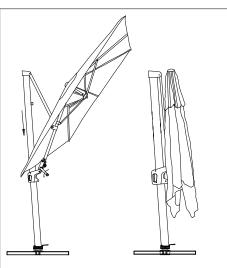
7. Push the slider button and pull it down to the middle position, then operating the crank counterclockwise. After the parasol closing, pull the slider down to the bottom position.
