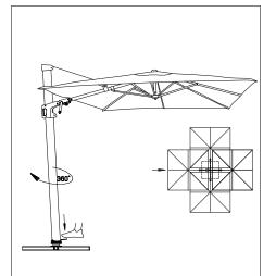
5. Press the rotating base pedal, the parasol could rotate  $360^{\circ}$ .
