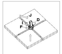
2. Assemble the rotating base(D) on the cross base and use the wrench(J) to screw the bolts(I) and washers(F).
