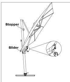
4. Push the button on the slider and boost the slider to the middle position, open the parasol completely by clockwise operating the crank, then boost the slider to the stopper.
